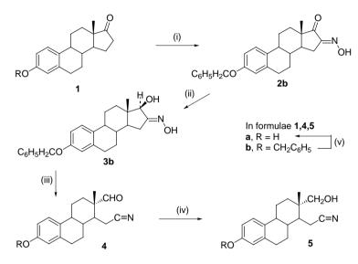
(i) (CH<sub>3</sub>)<sub>2</sub>CHCH<sub>2</sub>CH<sub>2</sub>ONO/(CH<sub>3</sub>)<sub>3</sub>COK/(CH<sub>3</sub>)<sub>3</sub>COH, 89.5%; (ii) NaBH<sub>4</sub>-1% aq. KOH/MeOH-CH<sub>2</sub>Cl<sub>2</sub>, 98%; (iii) TsCl/pyridine, 72%; (iv) NaBH<sub>4</sub>/MeOH, 96%; (v) H<sub>2</sub>-Pd/C/CH<sub>2</sub>Cl<sub>2</sub>-MeOH, 41% **4a**, 41% **5a**
